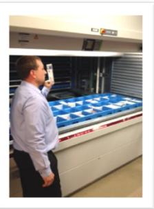
Parts manager, Stuart Sherre, showed us their state of art robotic parts bin system which stores around 85% of the dealership's parts inventory in a very small footprint. This frees up space in the service area and allows for automated parts inventory.
